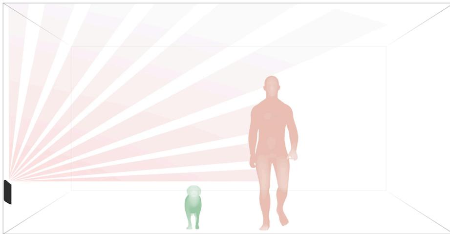
The placement of a MotionProtect Curtain also depends on the distance to a hub and whether there are any obstacles between the devices that may hinder the radio signal, e.g., walls, floor deck, or large objects in the room.
