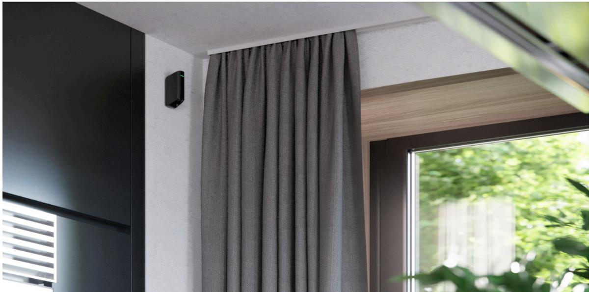
The effectiveness of the security system depends on detector placement. Choosing a location to install MotionProtect Curtain, consider the direction of the light filter and obstacles that may affect the detector's field of view and the radio signal transmission.
