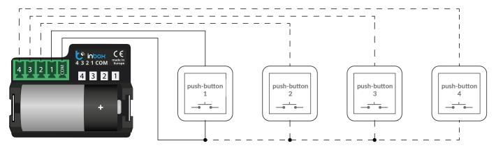
connect from one to four monostable pushbuttons
