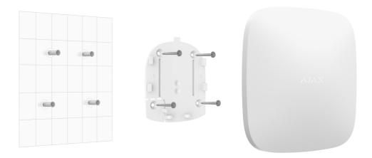
Before installing the hub, make sure that you have selected the optimal location and that it complies with the requirements of this manual.
